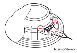
2. Remove the speaker grille (turn anti-clockwise). Fit the speaker into the cutout and secure the speaker using the screws (supplied).
